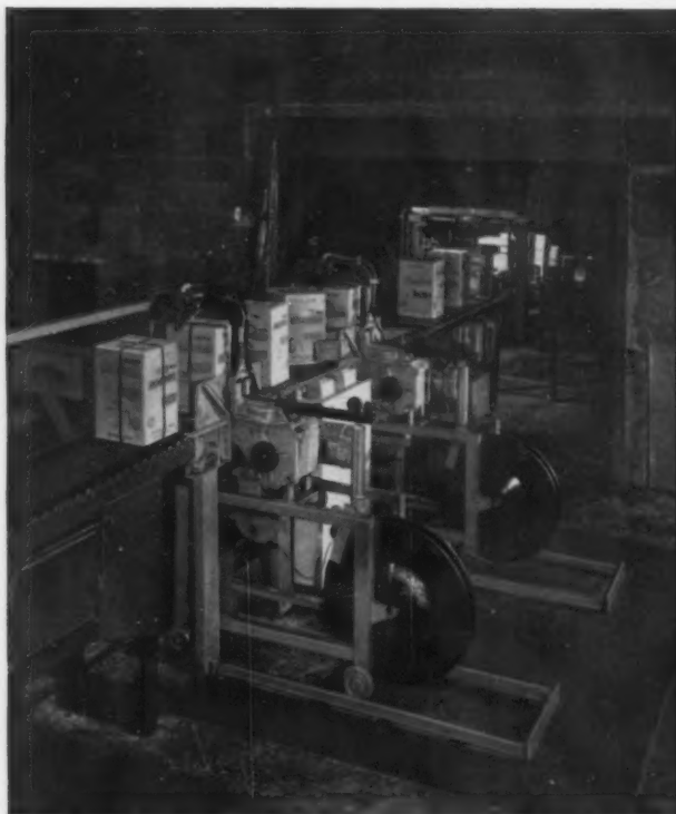
This completely automatic nail carton strapping machine has been in operation since 1955. Semi-automatic machines of this type have been in steel mill operation since 1946.
